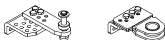
Fig. 9. Adjustable brackets for the BFT PHOBOS BT A25 and BFT PHOBOS BT A40 drive units.
