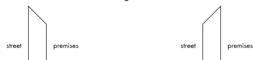
Fig. 21. Mitred finishing in the premises direction Fig. 22. Mitred finishing in the street direction. (standard).
